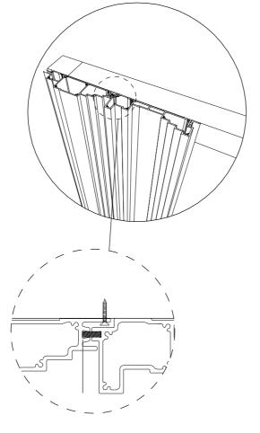
OptiDi should be screwed to the substructure with screws to adjust the width of the gap (a slit) using distance blocks provided as part of the order.
